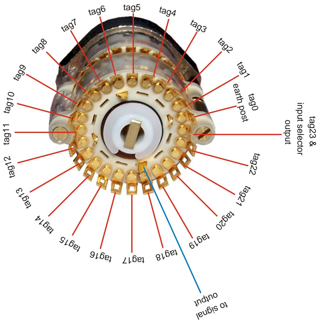
. Step 1: connect up the right channel transformer first, then take the switch apart and place the empty wafer at the top ready to solder the left channel transformer.
